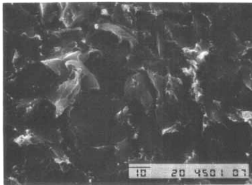
FIGURE 9 Scanning electron micrographs (500x) of the interfacial zinc (a) and polypropylene (b) sides of unaged anodized zinc (10% NaOH, 10 min., i = 30 \text{ mA/cm}^2 )/PP joints, (c) PP interfacial side of unaged grit-blasted zinc/PP joints.
